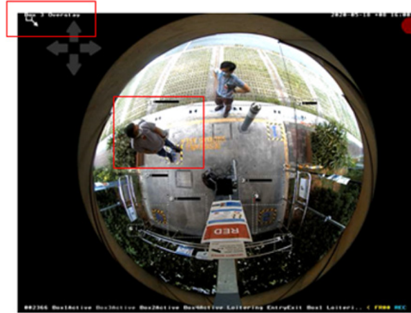
Figure 4: Overstay Monitoring (Exceeding time limit in box 3; voice message states: "Box 03 time limit exceeded, please leave.")
